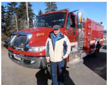
Mark Alley with GCI's new firetruck, a 2016 International 4400 Class A Pumper. This truck holds 970 gallons of water, 30 gallons of foam and can pump at 1250 gallons per minute.
